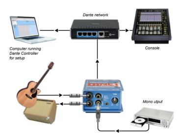
Note: When using the DAN-TX with an instrument and a stage amp, there is the possibility of encountering hum or buzz from a ground loop when using shielded Ethernet cables, due to the Dante network and the stage amplifier receiving power from different sources. There are two solutions to help alleviate the problem: 1. Use a CAT5e unshielded cable from the DAN-TX to the Dante Network. Or 2. Insert an isolator between the DAN-TX and the stage amp, such as the StageBug SB-6™.
