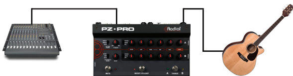
With the A+B switch engaged, the PZ-Pro can blend together two sources, such as a set of pickups and a microphone
