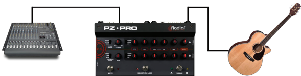
With only a single instrument connected to Input A, use the Toggle Footswitch to access the Level and EQ controls on channel B
